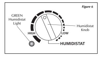
**NOTE:** The Humidifier will only turn on when the Humidistat is set to a high enough setting or when the room humidity is low enough.
