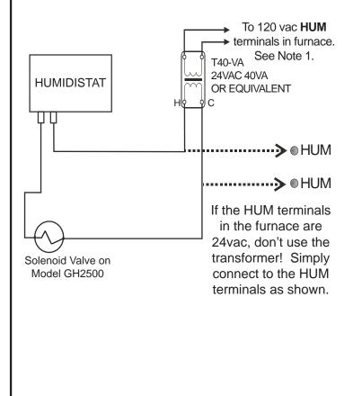
WIRING FOR MOST COMMON FURNACES
