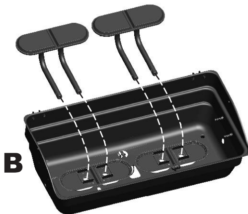
Correct burner-to-valve engagement
