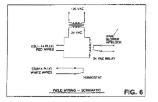
Connect field wiring as shown in Figures 5 & 6 to the red wires.
