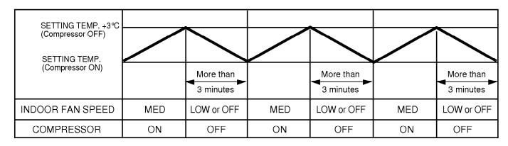
5. Auto Operation (Fuzzy Operation)The operation procedure is as following. (Cooling & Heating Model)
