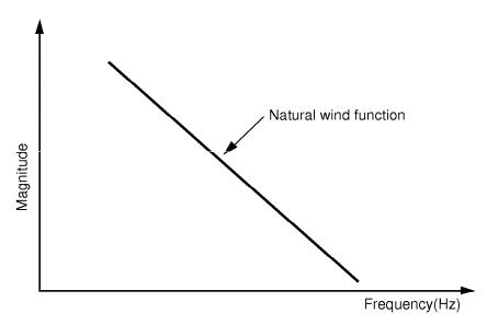
So as to make a similar Natural wind function, Indoor fan speed is shifted to high from low or reversely according to the CHAOS logic.
