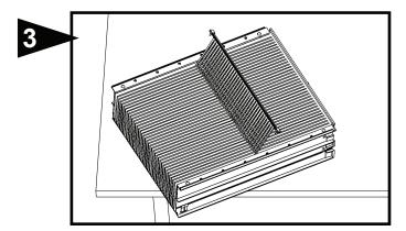
Install the plastic pleat spacers, being careful to insert one support finger between each pleat. Press each end of the pleat spacers down firmly to fully engage the media frame. Pleat spacers may snag on air cleaner cabinet if not pressed down below media frame rail.
