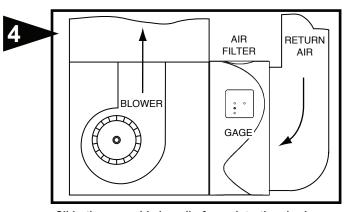
Slide the assembled media frame into the air cleaner cabinet. Be sure the airflow arrow on the media frame points toward the furnace blower. The plastic pleat spacers are always on the downstream side of the filter media. Attach outer cover.
