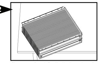
Place new media pack (Part No. 12758) onto the media frame. Slide media pack toward foam gasket. Line up holes in the cardboard strips with the holes in the media frame.
