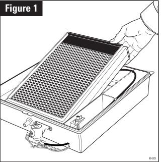
**3.** Position the two plastic hooks on the top of base along the top edge of the plenum opening. Push base up to engage the two hooks and sheet metal along the top edge opening. Push base in and slide down so that the bottom four hooks engage the sheet metal at the bottom edge of the opening. Secure base to opening using top three screw holes in housing. An additional hole is provided at the bottom for securing the base to the plenum. (**See Figure 2**)
