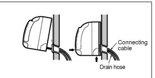
Press the lower left and right side of the unit against the Installation Plate until the lower hooks engages with their slots (sound click).
