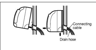
Press the lower left and right side of the unit against the Installation Plate until the lower hooks engages with their slots (sound click).
