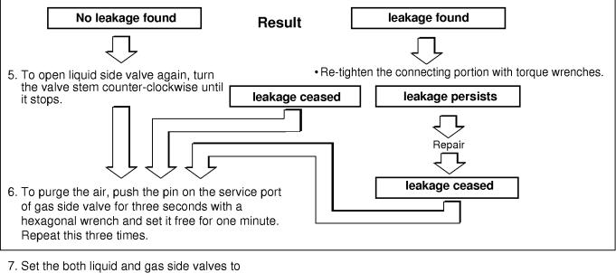
open position with the Hexagonal wrench for the unit operation.
