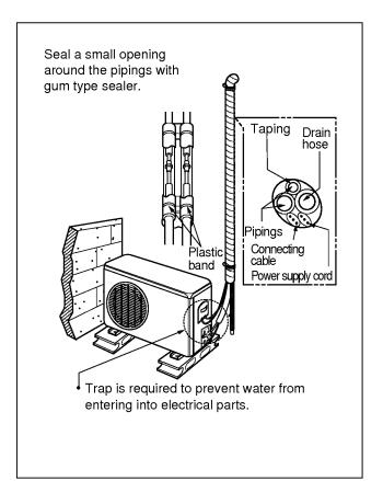
In case of the Outdoor unit being installed above position of the Indoor unit.
