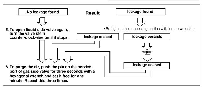
7. Set the both liquid and gas side valves to open position with the Hexagonal wrench for the unit operation.
