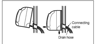
Press the lower left and right side of the unit against the Installation Plate until the lower hooks engages with their slots (sound click).
