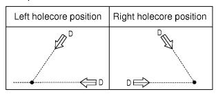
• Drill the Piping hole at either the right or the left and the hole should be slightly slanted to the outdoor side.
