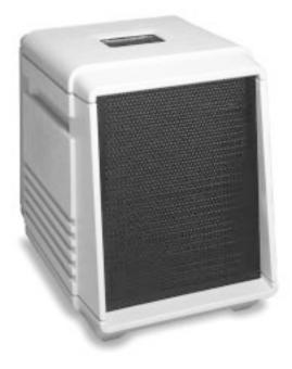
The Friedrich Electronic Air Cleaner is a self-contained console model consisting of a high voltage DC power supply, electronic cell, 3 speed fan, pre-filter and activated carbon post-filter in a rugged plastic cabinet.
