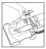
Replace filter into unit. Replace bottom filter cover by pivoting back onto cleaner from left to right.
