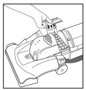
Remove the bottom filter cover by grasping the right edge and pivoting to the left.
