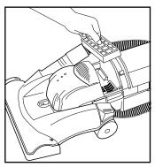
Pull filter frame from unit by pulling on tab in center.
