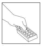
On some models, remove filter pad and shake to remove excess dust. If necessary this pad can be cleaned by vacuuming with another cleaner.
