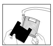
If necessary, the filter frame and foam filter can be rinsed in luke warm water and air dried. NOTE: The filter frame, foam and cover are not dishwasher safe.
