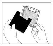
Remove foam from filter frame. Shake filter frame and foam filter to remove excess dust.
