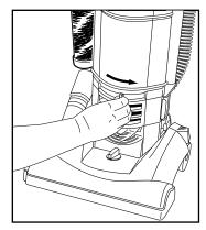
Replace dust cup lid, reposition in cleaner body and secure by moving lever from left to right.
