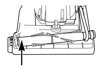
3. Remove the hood from the cleaner and check for a blockage in the brush roll area. Make sure the hose inlet is clear. If no blockage is found, continue to step 4.
