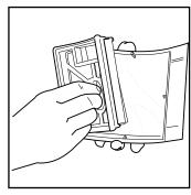
Remove filter frame from top filter cover.
