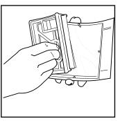
When dry, replace foam filter into filter frame.
