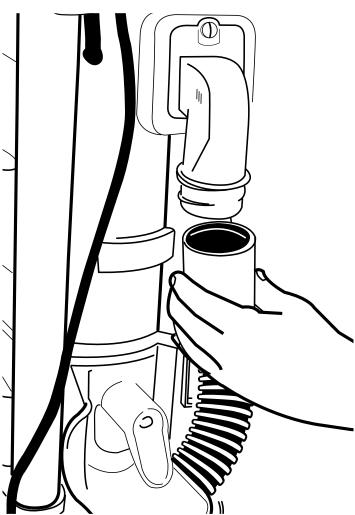
4. Twist the hose from the coupling elbow on the back of cleaner. Check for blockages at cleaner opening and in hose. If a blockage is found, clear the blockage.
