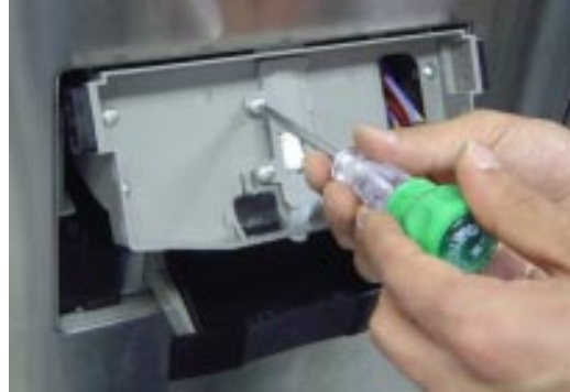
4) Unscrew 2 points and then remove connector-cover
