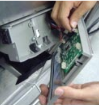
3) All harness have to be removed before separation of cover
