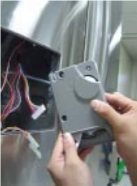
19) Pull motor box inside and then separate harness.
