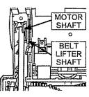
Place brushroll shutoff pedal in "Carpet" position. Slide belt onto motor shaft. Ensure to loop the belt around the belt lifter shaft.
