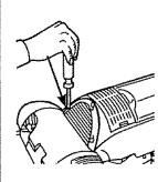
6. Snap lens cover back into place and secure the headlight lens by replacing the two screws.
