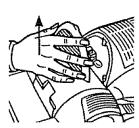
4. Insert flat blade of screwdriver into slot at top of the lens. Lift the lens cover to remove.
