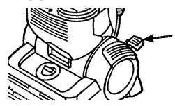
Rotate the handle and adjust it to the desired position for (A) storing the upright, (B) operating the cleaner, and (C) to clean under furniture. **NOTE:** Rotating brush could cause area rug fringe to become tangled within cleaner. Use caution when vacuuming any rugs with fringe.
