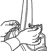
2. Push handle plug onto the front of cleaner. Insert the one (1) screw into the back of the handle and tighten, making sure the handle plug is secure.
