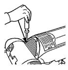
**3.** Remove the two (2) screws from the lens cover.
