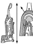
Cleaner must be in its upright position to raise brushroll from floor. Remove the hose from the tool caddy.
