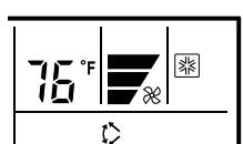
Press the vertical airflow direction and swing button for 2 seconds or more to select or stop swing operation. The vertical swing display appears during swing operation.
