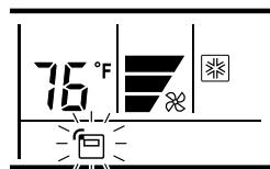
Press the THERMO SENSOR button to select whether the room temperature is detected at the indoor unit (remote sensor) or the remote controller.
