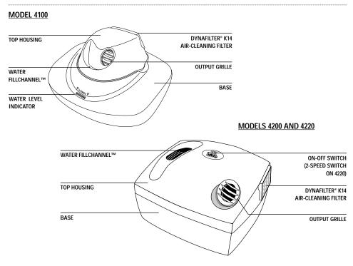
The Kaz HealthMist\* 4100, 4200 and 4220 models produce a cool mist through revolutionary new cyclone technology. The motor-driven impeller draws up water through a pickup tube. Centrifugal force throws the water through a screen into the vortex chamber, breaking up the water into a superfine, cool mist.
