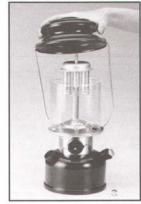
Tie mantle around groove in burner and cut off ends of string 1/4" (.64 cm) from knot.
