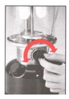
Adjust fuel valve to desired brightness. To clean generator tip, turn fuel valve from high to off to high several times.
