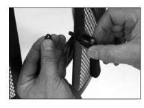
**5d.** Tighten the "jam nut" with a wrench.
