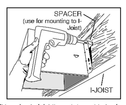
nails. Screw or nail housing to joist through lowest holes in each mounting flange, then through highest holes. NOTE: Mounting to I-JOIST (shown) requires use of SPACERS (included) between the highest hole of each mounting
