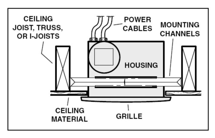
Housing mounted directly to joists, trusses, or I-joists.
