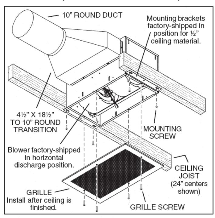
Factory-shipped unit installed in <u>new</u> construction.
