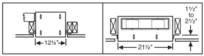
Mounting brackets mounted to outlet sides of housing. (Outlet perpendicular to joists.)
