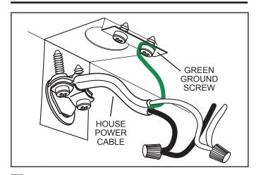
Gonnect House Power Cable to range hood wiring - BLACK to BLACK, WHITE to WHITE, and GREEN or BARE WIRE to GREEN Ground Screw.
