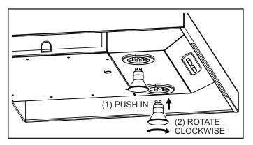
Install <u>Halogen Bulbs</u>. Use 120 V, 50 W, shielded halogen bulbs - MR16 or PAR16 with GU10 base. Purchase bulbs separately.
