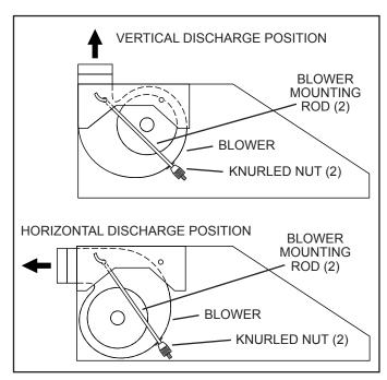
4 Blower is shipped in Vertical Discharge Position.
