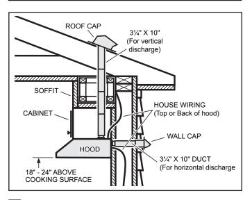
Determine whether hood will discharge vertically or horizontally. For vertical or horizontal discharge, run ductwork between the hood location and a roof cap or wall cap. For best results, use a minimum number of transitions and elbows.
