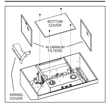
Remove the <u>Aluminum Filters</u>, <u>Bottom Cover</u>, and <u>Wiring Cover</u> from the hood.
