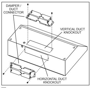
Remove <u>Vertical Duct Knockout</u> or <u>Horizontal Duct Knockout</u> and attach <u>Damper / Duct Connector</u> with two (2) screws (supplied).
