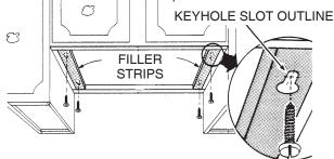
6. Screw the four supplied screws for mounting the hood into the exact center of the narrow end of the keyhole slots marked underneath the cabinet. Allow 3/8" of the screws to project, so the hood can be fitted into place.
