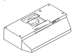
**Round Vented** — 7" vertical. Remove knockouts #① and #② exposing duct collar. Go to "Planning Ductwork Installation".
