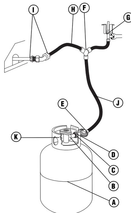
6. Check each place listed (A–K) for growing bubbles which indicates a leak.
