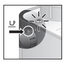
Once the milk is frothed, put a cup underneath the filter holder. Turn the knob to the "Coffee" position.
