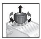
■ Unscrew the boiler cap. Measure out the right amount of water for your needs and pour it into the water tank. For instance: an espresso-sized cup (small cup for strong coffee) = 1 to 2 oz (25 to 50 ml). A standard-sized cup (for milder coffee) = 3 to 4 oz (75 to 100 ml). Up to 4 espressos or 2 standard cups can be made at one time, without adding additional water to the tank.
