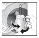
■ When the steam starts coming out of the nozzle, immerse the nozzle in the pitcher of milk and make circular movements going up and down to froth the milk. It is important not to have the nozzle touch the bottom of your pitcher.
