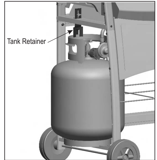
Correctly Installed LP cylinder.
