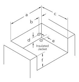
**Note:** Insulated jacket required for all grills installed into a cumbustable enclosure.
