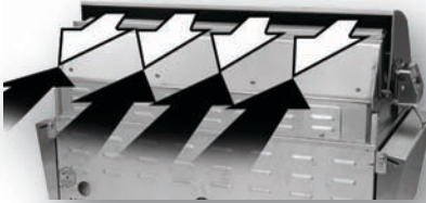
Fig 3 - Wind hitting the back of the grill can disrupt proper exhaust.
