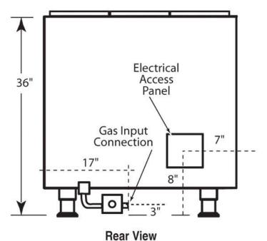
Electrical Requirements: 50 Amp Circuit (Equipped with 6ft. power cord)
