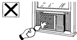
Do not splash water or detergent into the unit's body openings.
