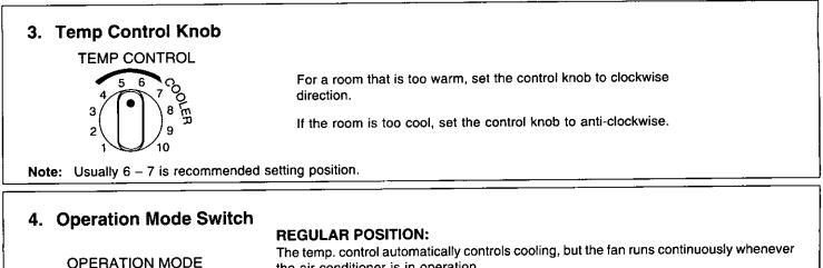
The temp. control automatically controls cooling, but the fan runs continuously whenever the air conditioner is in operation.
