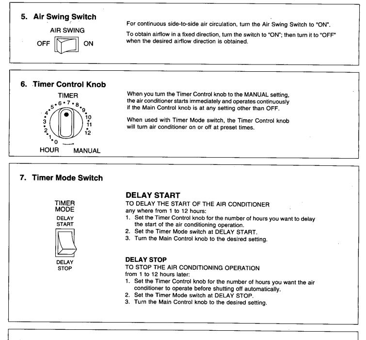
Note: If the unit is turned OFF and immediately on again, an automatic protection device will prevent restart of the compressor for approximately 3 minutes. <u>THIS IS NORMAL, LEAVE THE SWITCH ON AND OPERATION WILL RESUME</u> <u>AUTOMATICALLY WHEN THE PROTECTION DELAY IS COMPLETED.</u>
