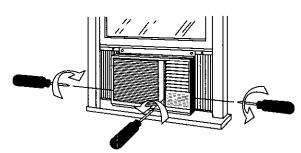
3. Pull the front grille towards yourself from the bottom first, lift up and remove it.
