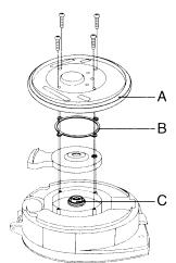
Remove lid, unscrew 4 tapping screws and the lid cover. Exchange the gaskets and the the lid cover back and secure with the tappi
