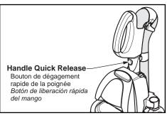
> Press the handle quick release button on the wand to remove the handle to use tools on the handle.
