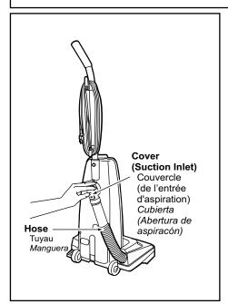
The hose located on the back of the vacuum cleaner carries the dirt from the nozzle up to the dust bag. If the hose should become clogged:
