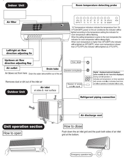
Lightly push both sides of the air inlet grid at the botton and pull it to this side till a resistance is felt.
