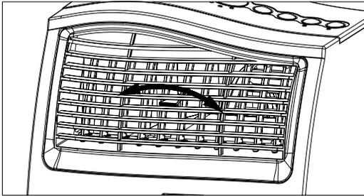
Adjust louver on the air vent horizontally to control air flow direction.
