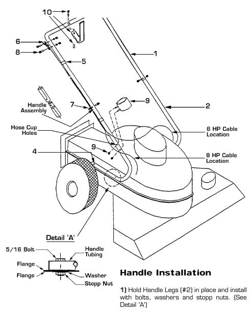
**2)** Install Handle 'U' (#1) making sure Remote Control holes on 'U' are on right side as you push the machine.
