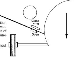
**Note:** Pull litter vac backwards before rotating the T-Handle to re reverse front wheels allowing full movement of baffle plate
