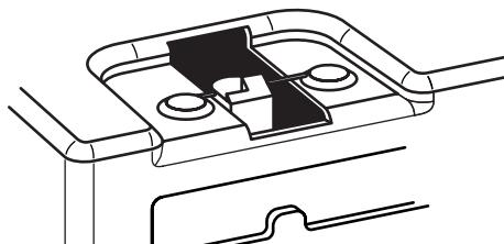
You can set the adjustable Water Level Float at the "high" or "low" position. Both settings will turn off the dehumidifier automatically. To adjust water level, push float left or right until it snaps into place.
