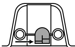
"Low" setting: Slide Water Level Float to "low" position - right side of opening - to make the bucket lighter to carry. The dehumidifier will shut off automatically when bucket is  $\frac{1}{2}$  full.
