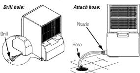
**Use a floor drain.** The unit can also be placed over a floor drain. Using a drill, make a hole at the end of the nozzle located on the lower left side of the bucket.
