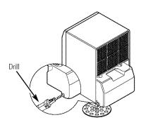
**NOTE**: The nozzle cannot be fixed after puncture. Use an ordinary garden hose cap (not included) to reclose if necessary.
