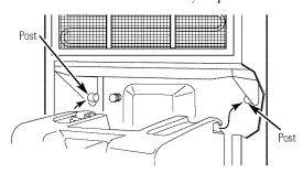
Make sure the bucket is locked securely in place by pressing down on the upper back edge of the bucket. It will be firmly seated when properly installed.
