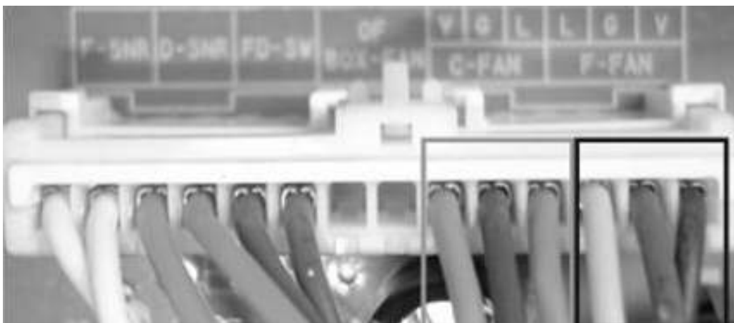
CON7 CON7 C-FAN F-FAN PIN 9, 10, 11 PIN 12, 13, 14 GY, BN, SB YL, PR, BL
