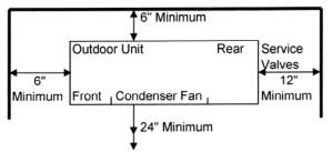
Install the Outdoor unit on a Condenser Pad or if a Heat Pump use feet to raise unit up approx 6" to allow for defrost to drain away
