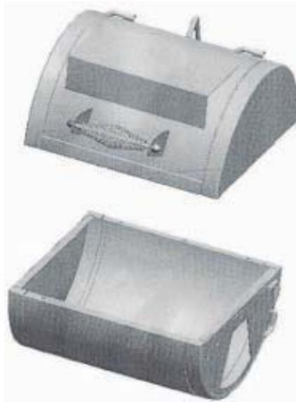
**10** Attach the Firebox Assembly to the Smoker Chamber - match the heat Passage Opening of the both parts. NOTE: the Heat Deflector is to be attached IN the Smoker Chamber using the top (2) bolts. Use (8) M10X25 long Hex Head Bolts and M10 Flat washers, through the two assemblies and secure with M10 Flat Washers, M10 Lock washers and M10 Hex Nuts. Tighten all bolts.
