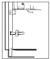
Failure to align the "V"s properly or to latch the drawer to the door may cause the compactor to not function properly.
