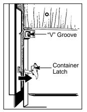
• Finally, use the container latch to completely close the door. This will pull the door guide "V" snug in the "V" groove in the drawer flange and tightly grasp the bag.
