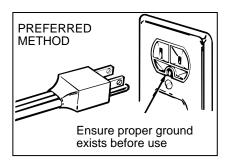
This appliance is equipped with a cord having an equipment grounding conductor and a grounding plug. The plug must be plugged into an appropriate outlet that is properly installed and grounded in accordance with local codes and ordinances.
