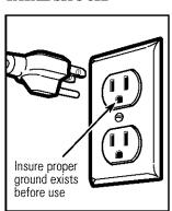
The power cord of this appliance is equipped with a 3-prong (grounding) plug which mates with a standard three-prong (grounding) wall receptacle to minimize the possibility of electric shock hazard from this appliance.
