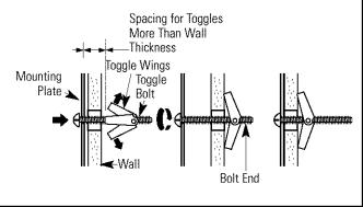
Place the mounting plate against the wall and insert the toggle wings into the holes in the wall to mount the plate.
