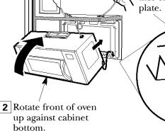
Insert a self-aligning screw through right top center cabinet hole. Temporarily secure the oven by turning the screw at least **two full turns** after the threads have engaged. (It will be completely tightened later.) Be sure to keep power cord tight. Be careful not to pinch the cord, especially when mounting flush to bottom of cabinet.
