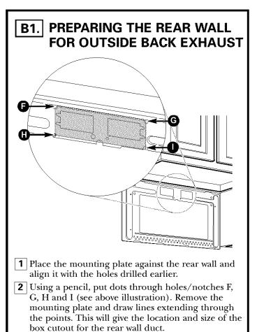
Use a saw (saber or keyhole) to cut out the opening.Place the microwave in its upright position with the
