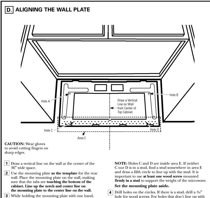
hole for wood screws. For holes that don't line up with a stud, drill a %" hole for toggle bolts.
