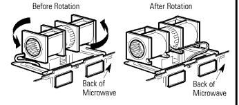
Gently remove the wires from the grooves.
