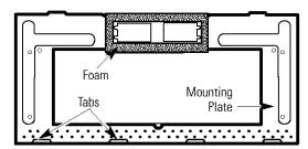
Attach the other 28" foam tape to the front of the mounting plate around both of the exhaust openings where it will touch the microwave.
