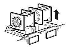
Roll the blower unit 90° so that fan blade openings are facing toward the front of the microwave.
