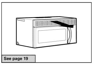
A Charcoal Filter Accessory Kit is required for the nonvented exhaust. (See your Owner's Manual for the kit number.)
