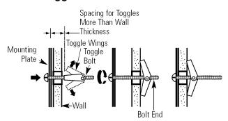
**3** Place the mounting plate against the wall and insert the toggle wings into the holes in the wall to mount the plate.
