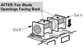
CAUTION: Do not pull or stretch the blower unit wiring. Make sure the wires are not pinched.
