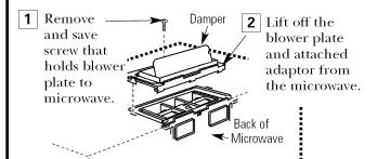
Slide exhaust adaptor to one side and remove it. **NOTE:** The exhaust adaptor with damper is not needed for recirculating models. You may want to save them for possible future use.
