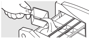
Insert in forward position for liquid detergent
